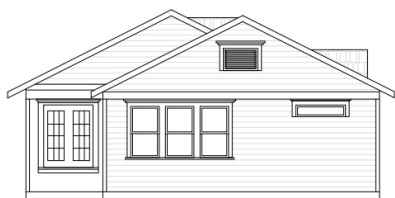
EXISTING SOUTH EXTERIOR ELEVATION SCALE: 1/4"=1'-0"
